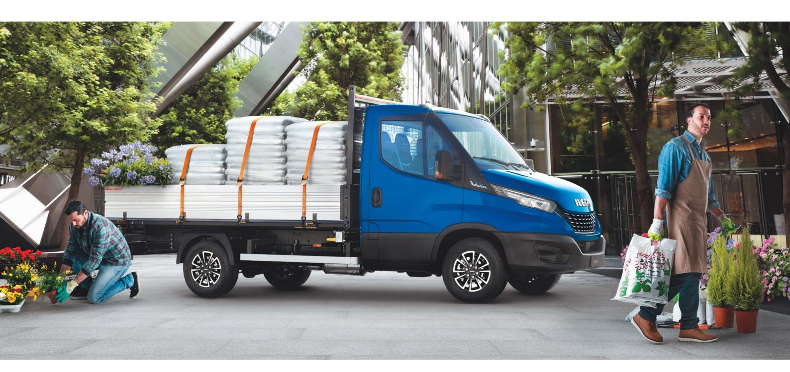
**Carry a bigger payload** with the high-performance front suspension, which raises the maximum permissible load. You can count on a front axle maximum load capacity of up to 1900 kg on the 3.5-tonne models featuring the lighter, strong QUAD-LEAF suspension, or even higher, as much as 2700 kg, if you opt for a twin wheel model with the QUAD-TOR suspension.
